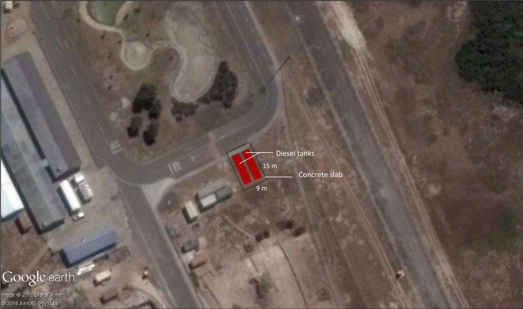
Figure 1: Illustration of the layout of the proposed diesel tanks at the Ekhaya site.
